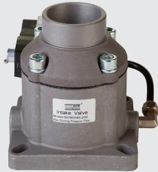
The SCR suction valve is a high quality key component which brings the compressor on and off load and has an expected service life of over 2 million cycles. The longevity and reliability of this valve is due to no gap needing to be completely sealed, therefore eliminating problems such as deteriorating cup seals and diaphragms.
