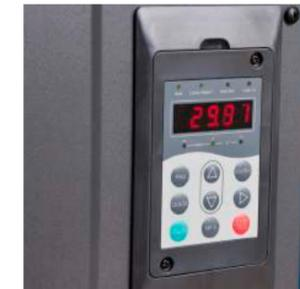
The Inovance inverter has a massive 30-100% variable range which converts AC to DC to control the new IPM motor. According to your air consumption the inverter will automatically adjust the IPM motor to suite your air demand while keeping a stable pressure of 0.1bar.
