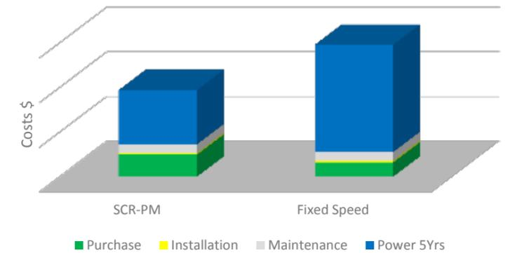
Chart compares the costs of owning a fixed-speed 45kw compressor producing 7.2m<sup>3</sup>/min (254cfm) compared to using a high efficiency 7.2m<sup>3</sup>/min (254cfm) SCR EPM 37kw VSD compressor over just a five-year period, where the fluctuating air demand in a typical workshop, equates to a loaded run time of 30% of the day.
