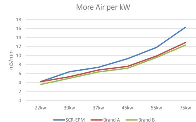
SCR have added a new high efficiency compression airend to the EPM series which delivers 10-15% more air. The size of the airend has also been increased and reaches optimum flow at significantly lower revolutions.
